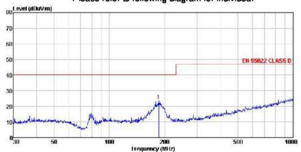
Site : 3m chamber Condition : EN 55022 CLASS B 3m VULE9163-20:3M VERTICAL EUT :
